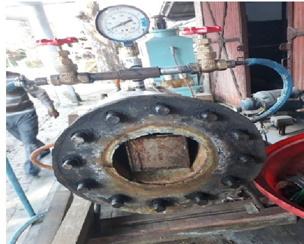
Plate 2: Pressure Chamber Loaded with Charge
